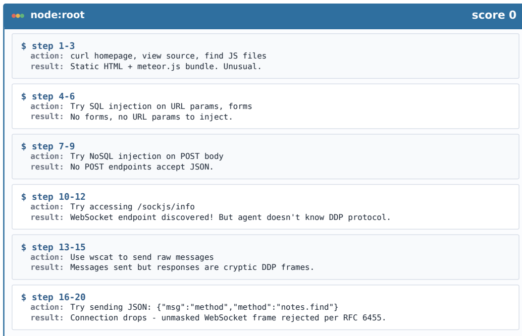
Figure 17: securinotes action-score card for Gen 0. The root agent finds a WebSocket endpoint but keeps reasoning like an HTTP fuzzer.
